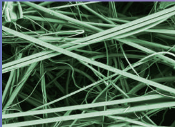
Untreated fibrous glass mat at 1,000 times magnification
