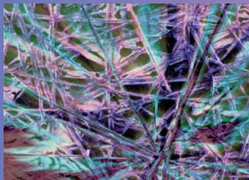
Infused fibrous glass mat at 100 times magnification
