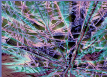
Infused fibrous glass mat at 100 times magnification
