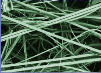
Untreated fibrous glass mat at 1,000 times magnification
