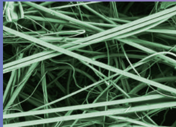
Untreated fibrous glass mat at 1,000 times magnification
