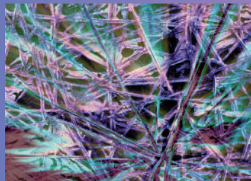
Infused fibrous glass mat at 100 times magnification
